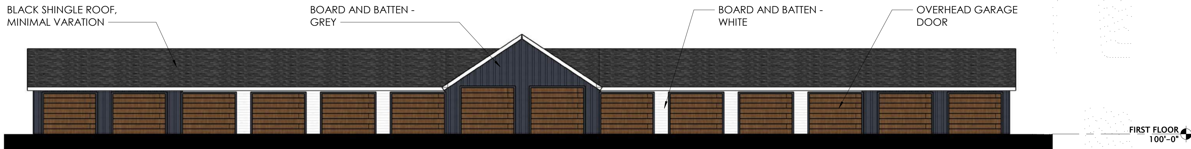
6 SOUTH GARAGE ELEVATION 1" = 10'-0"
